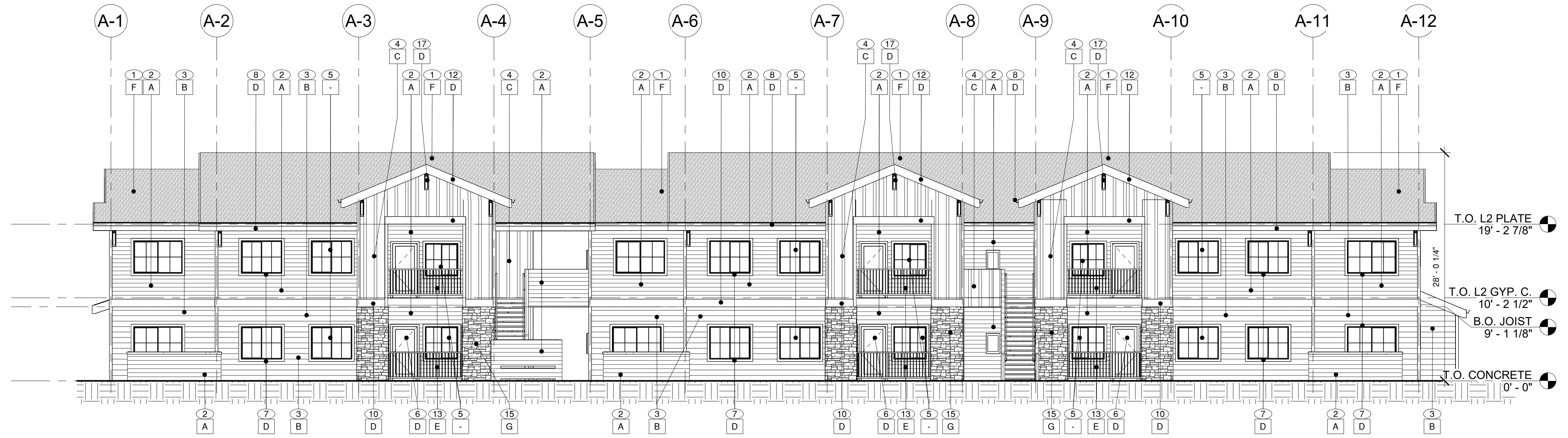
1 FRONT ELEVATION - BLDG. TYPE A 1/8" = 1'-0"
